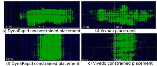
Fig. 12: Visualization of Vivado and DynaRapid placement density for the video\_filter benchmark. (a) DynaRapid placement. (b) Vivado placement in the same region. (c) Vivado’s manually obtained minimum footprint. (d) DynaRapid placement constrained to Vivado’s minimum footprint.
