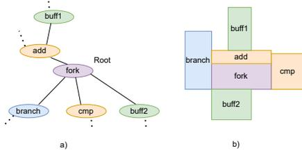
Fig. 8: Greedy Placement. (a) *fork* is the first unit placed because it has the largest number of connections to other units. (b) Components are placed in topological order starting from the *fork*, using the footprint that allows the closest placement to the centre and, in the case of ties, the tallest footprint.
