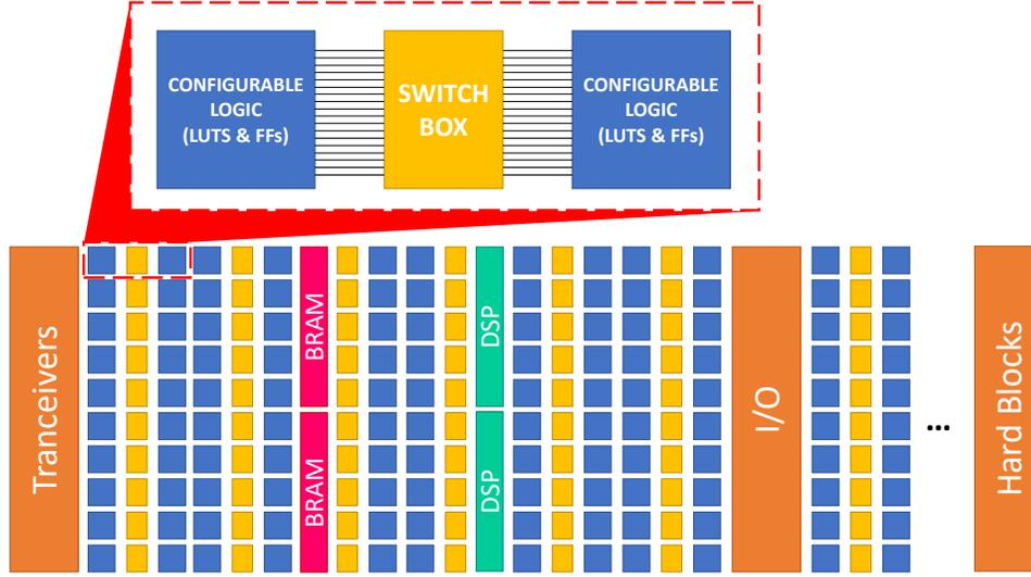
Fig. 2. FPGA with columnar resources.
