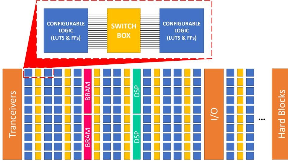
Fig. 2. FPGA with columnar resources.
